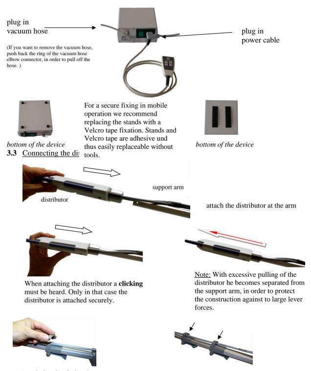
Attach the plug-in brackets.
