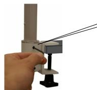
Tighten the upper grub screw (M6x6) so that the foot of the support arm presses firmly against the clamping device.
