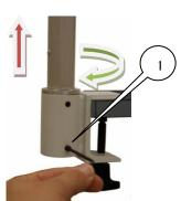
The threaded hole at the foot of the support arm must match the lower threaded hole of the clamping device.
